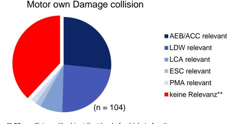
\*\* 28 x collision with object (lost load of vehicle in front) 4 x burst tires 3 x v > 130 km/h 3 x aquaplaning
