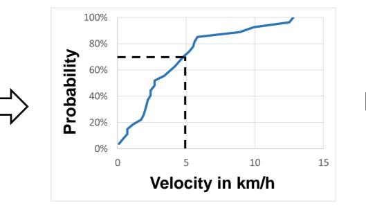
At a velocity of 5 km / h up to 70 % of collisions avoidable
