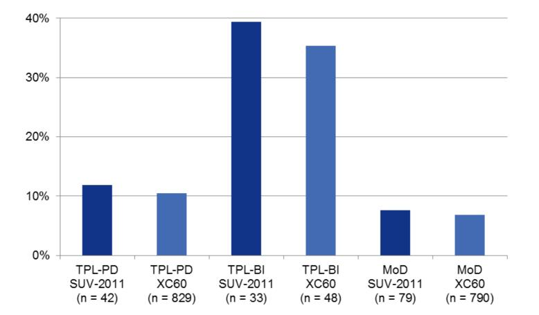
• Volvo City Safety seems to be effective by reducing the frequency of rear end collisions
